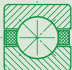
Axial-Ball thrust bearing PBAC 9,525 x 9,525
